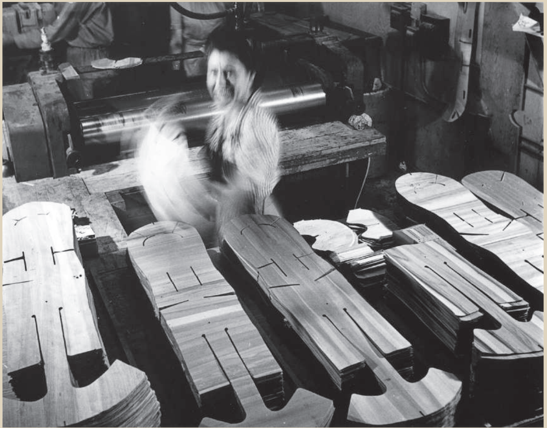
Manufacturing the Eames Moulded Plywood Splint from component parts, 1943. Photo: ©2017 Eames Office, LLC (eamesoffice.com).
